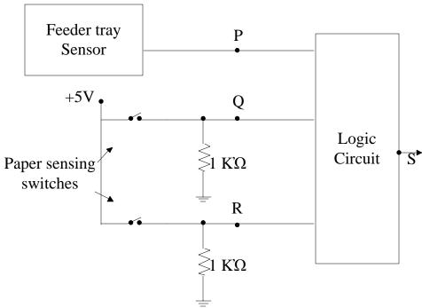
The S output will be a logic 1 whenever P=0 because this indicates no paper in the paper feeder tray. S will also be a 1 for the two cases where Q and R both indicating a paper jam.
